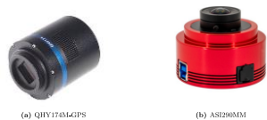
図 4: (a) QHY174M-GPS (made by QHY) is a mainstream camera among overseas occultation observers. (b) ASI290MM (made by ZWO) is popular among Japanese occultation observers because of its low price. But this ASI290MM has no GPS function. To compensate for the lack of GPS function, it is necessary to use a GPS module at the same time (see text for details).
