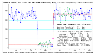
図 8: We analyzed the video shown in Figure 6, and then fit the diffraction simulation model to the light curve of the star occulted by the asteroid to obtain the most likely value of the event time. As a result, we found that 17h43m 22.785 \pm 0.021s was the most likely value of the event time. This means that the event occurred 0.081s before the timestamp of 17h43m 22.866s, which is the timestamp of the frame in which the faint star image was seen.
